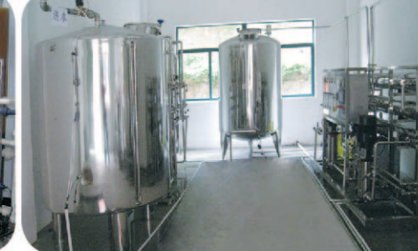
上海瑞耳高泰医疗器械有限公司(2m 3 /h二级反渗透纯化水设备) Shanghai Realgold Medical Co.,Ltd (2m 3 /h two stage Reverse Osmosis equipment)
