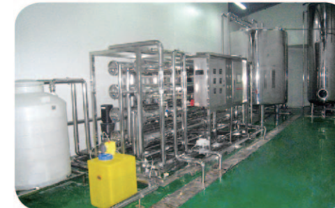
浙江楠溪江啤酒有限公司(40m 3 /h反渗透纯净水设备) Zhejiang Nanxriver brewery Co.,Ltd (40m 3 /h Reverse Osmosis equipment)
