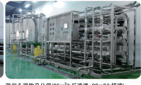
温州永强饮品公司(25m 3 /h反渗透+20m 3 /h超滤) Wenzhou Yongqiang Drinking Products Company(Capacity 25m 3 /h Reverse osmosis +20m 3 /h Ultrafiltration equipment)
