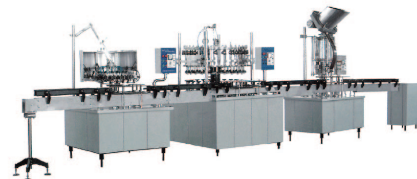
时产2000-4800瓶500ml/瓶冲洗、灌装、旋盖流水生产线 2000-4800b/h linear water filling production line
