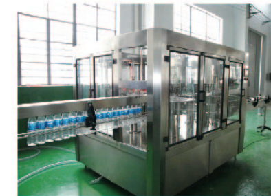
时产5000-10000瓶500ml/瓶冲洗、灌装、旋盖三合一瓶装生产线 5000-10000b/h 3 in 1 water filling production line
