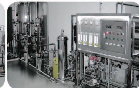
哈药集团世一堂(2m 3 /h 二级反渗透纯化水设备) Harbin Pharmaceutical Group Shiyitang (Capacity 2m 3 /h two stage Reverse Osmosis equipment)
