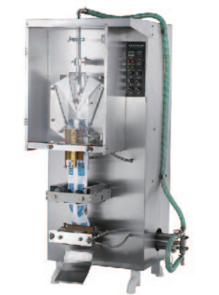
时产1600-2000袋500ml/袋液体包装机 (适合饮用水、酱油、饮料等软性液体) 1600-2000 bags/hour sachet water packing machine
